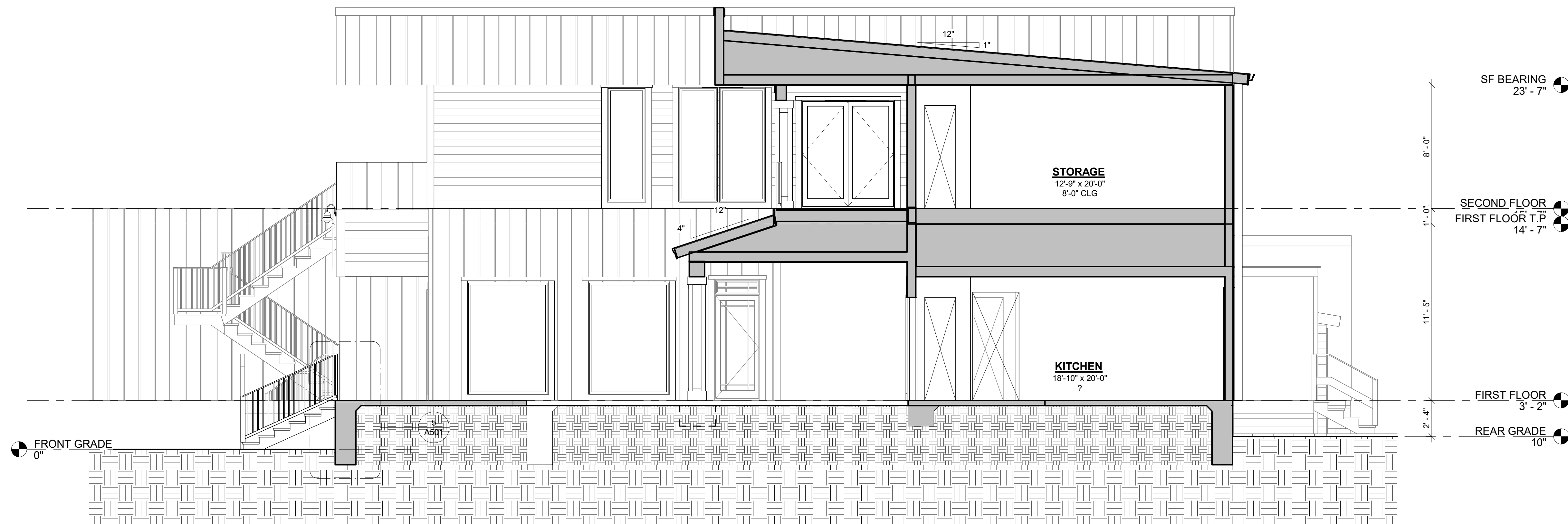
BUILDING SECTION @ BREEZEWAY & RECEIVING CAFE SIDE ② 1/4" = 1'-0"
