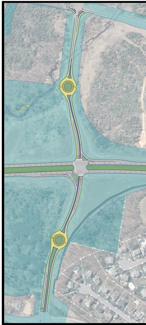
Figure 4. Example Bowtie Intersection (Provided by Virginia DOT)
