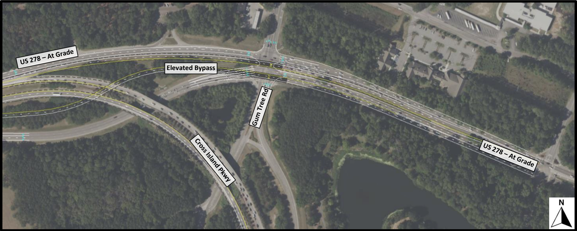
Figure 10. Example of Elevated Bypass - 04
