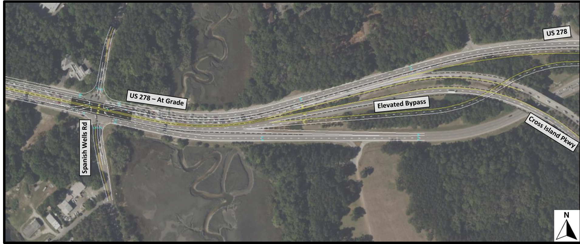
Figure 9. Example of Elevated Bypass - 03
