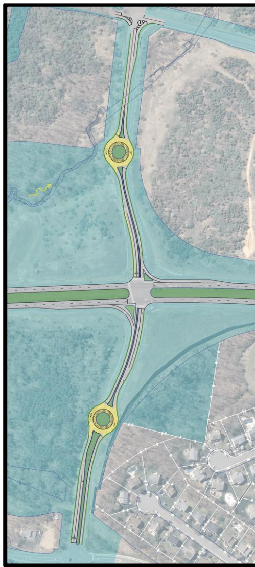
Figure 4. Example Bowtie Intersection (Provided by Virginia DOT)
