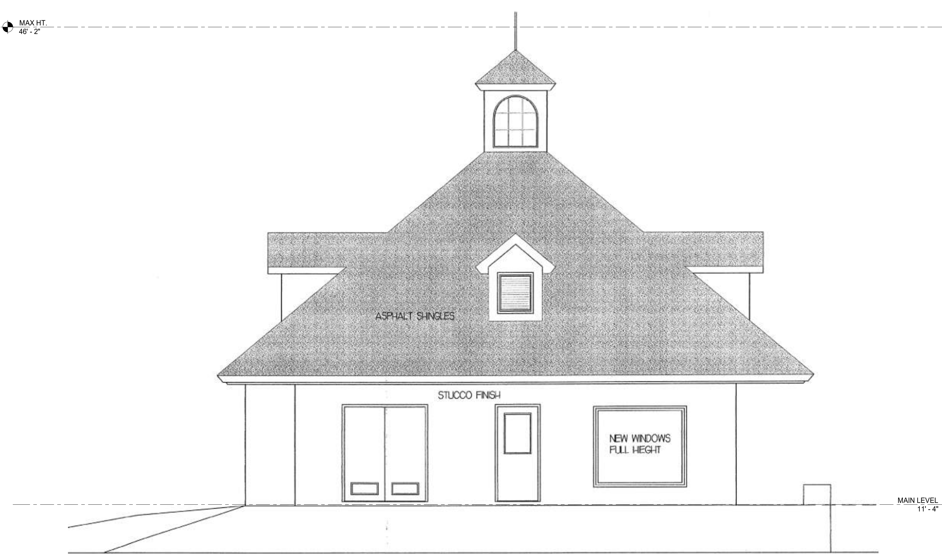
2 SW ELEVATION - EXISTING 1/4" = 1'-0"
