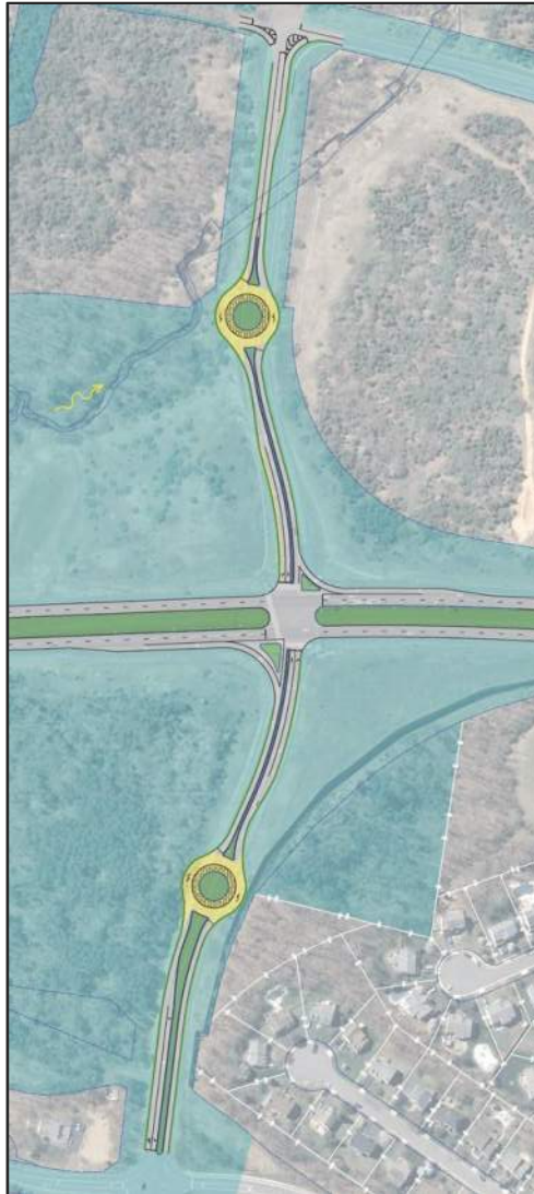
FIGURE 4. EXAMPLE BOWTIE INTERSECTION (PROVIDED BY VIRGINIA DOT)
