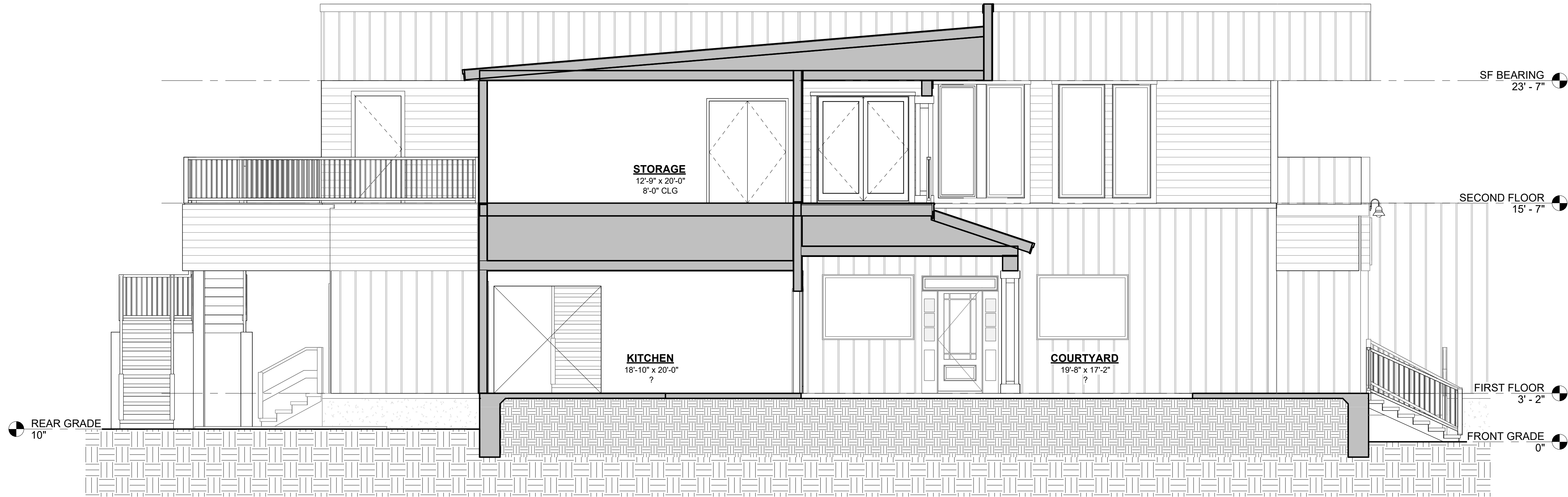
BUILDING SECTION @ BREEZEWAY & RECEIVING ① 1/4" = 1'-0"
