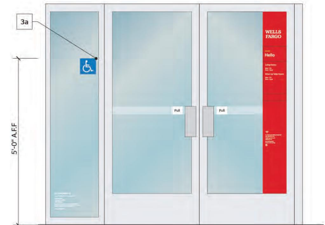
4a Elevation — ADA Decal Placement Scale: NTS
