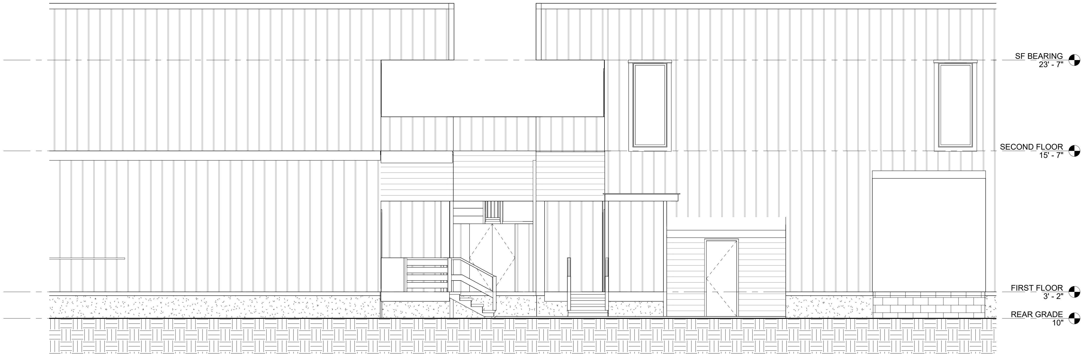
② AS-BUILT REAR ELEVATION 1/4" = 1'-0"
