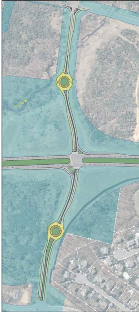
FIGURE 4. EXAMPLE BOWTIE INTERSECTION (PROVIDED BY VIRGINIA DOT)
