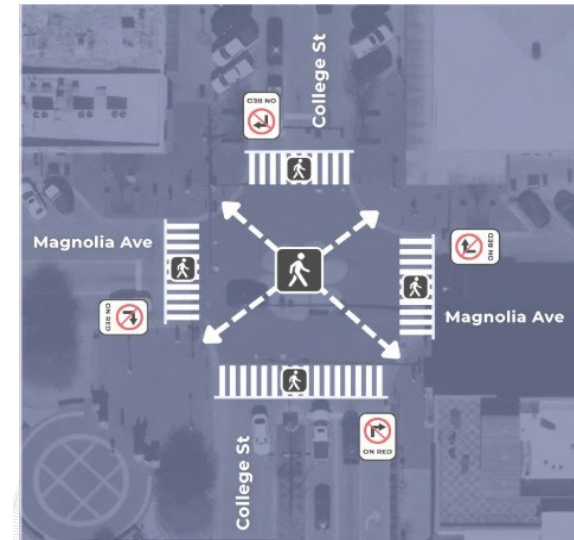
Phase 1: Pedestrians only Pedestrians are given a minimum 3–7 second head start entering the intersection.
