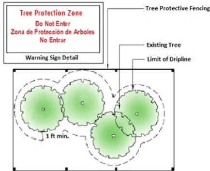
Figure 16-6-104.J.2: Tree Protective Fencing and Signage.
