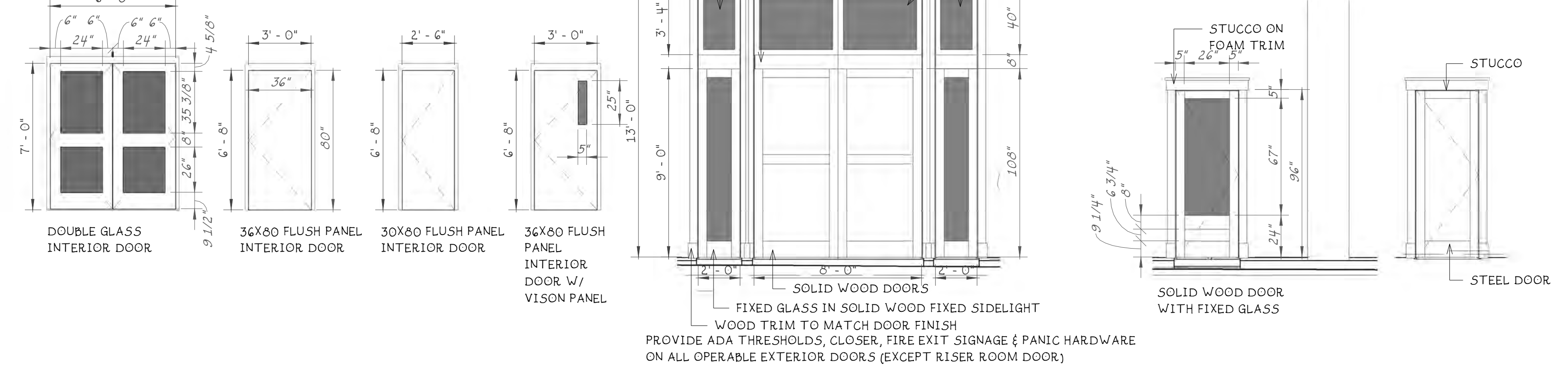
① INTERIOR DOOR TYPES 1/4" = 1'-0" ① - ENTRY DOOR 1/4" = 1'-0" ② SIDE DOORS 1/4" = 1'-0" ③ RISER ROOM DOOR 1/4" = 1'-0"
