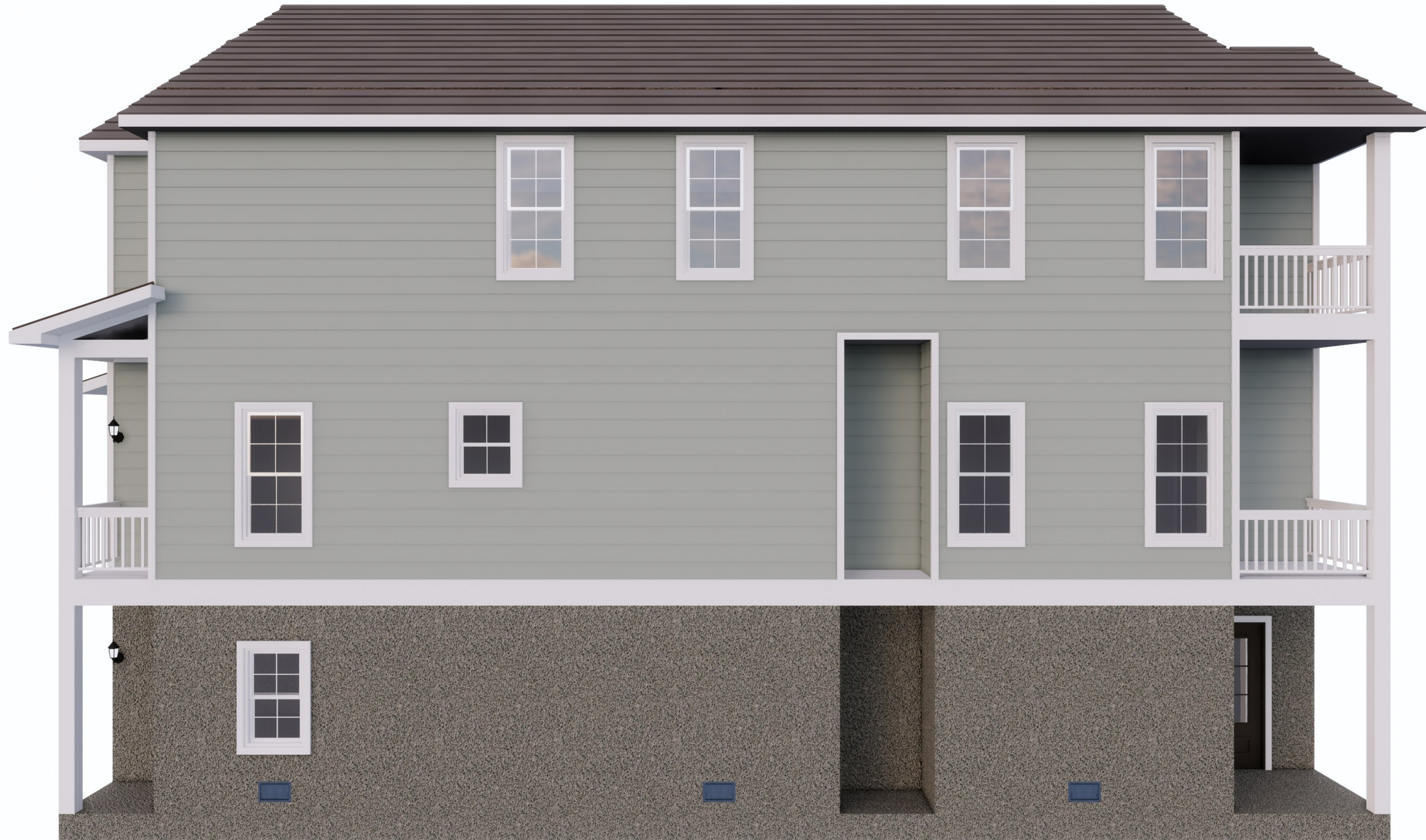
ELEVATION SHOWING TYPICAL FLOOD VENT LOCATIONS
